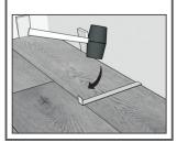
2. Lock short end of plank by inserting tongue into groove at an angle and drop in place Continue to the end of the first
