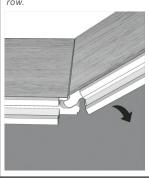
5. Lock long edge of plank by inserting tongue into groove at an angle and drop in place. Slide plank toward end of previously installed plank until the tongue just touches the groove.
