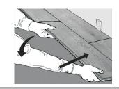
8. Tap end of plank with rubber mallet and tapping block to lock ends of planks together. Remove bridge and continue towards wall until installing the final plank in the row. Be sure to tap on edge of tapping block so as not to damage locking profile.
