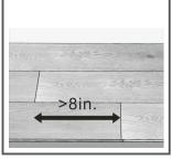
7. Attach a scrap piece of floor to bridge gap between ends of planks.
