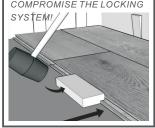
9. Use rubber mallet and pull bar to lock final piece in row. Insert spacer at end of row. Continue installation to final
