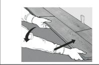
8. Tap end of plank with rubber mallet and tapping block to lock ends of planks together. Remove bridge and continue towards wall until installing the final plank in the row. Be sure to tap on edge of tapping block so as not to damage locking profile.
