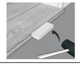
12. Use rubber mallet and pull par to lock short end of plank.
