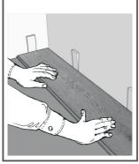
4. There must be at least 8" between plank end joints on adjacent rows.
