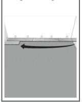
6. IMPORTANT! Use rubber mallet and tapping block to tap long edge of plank to ensure a tight fit. ANY GAPPING CAN COMPROMISE THE LOCKING
