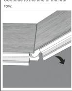
5. Lock long edge of plank by inserting tongue into groove at an angle and drop in place. Slide plank toward end of previously installed plank until the tongue just touches the groove.
