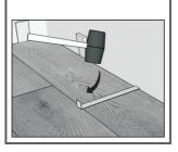
2. Lock short end of plank by inserting tongue into groove at an angle and drop in place Continue to the end of the first
