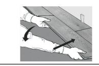
8. Tap end of plank with rubber mallet and tapping block to lock ends of planks together.
