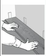
4. There must be at least 8" between plank end joints on adjacent rows.
